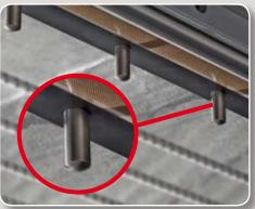
**Waste handling:** An optional trim removal and collection system rounds out our vacuum chamber packaging machine. It features an automatic cutting system that trims the excess material while the product is held tightly in place (via flexible expanders and spring powered pins) and then disposes the material into a 120-liter stainless steel container.
