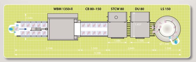
Above: Inline shrink packaging, featuring our Chamber Belt Machine WBM 1350-II, Conveyor Belt CB 80, Shrink Tunnel STCW 80-L, Dryer DU 80-L and Turntable LS 150.
