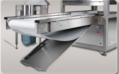
Conveyor belt loosens with the push of a button: When it comes time for sanitation, operators can gain full access to the conveyor belt and machine's decking with the push of a button.
