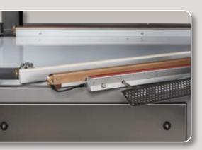
Secure seals: Our intelligent Thermo Controlled Heat Sealing System (TCH-II) guarantees secure sealing results. Optimum sealing temperatures are reached through constant and precise control. Overheating of the seal bars and the packaging material is avoided due to the precise temperature regulation. Sealing parameters for the TCH-II and reliable bi-active sealing can be adjusted according to the packaging material.
