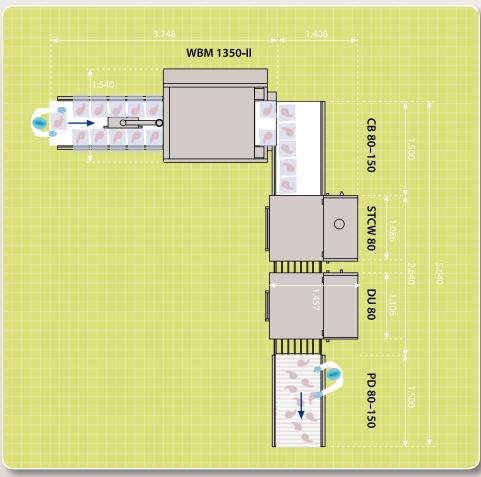
Compatible with any production line: Our high-capacity WBM 1350-II is the ideal packaging machine for any shrink packaging application. Designed for flexibility, the WBM 1350-II completes any shrink packaging line, featuring our Shrink Tunnel STCW, Dryer DU, variable Conveyor Belts CB, Product Depot PD or Turntable LS.
