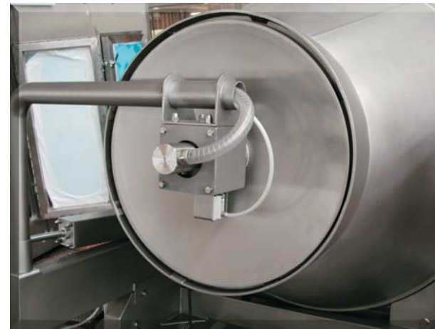
Automatic cover opening with integrated vacuum system (option)
